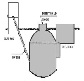
Figure 2 – Chinese Model Biodigestor (BENINCASA, 1990)
