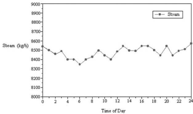
Figure 3 – Process Steam Consumption (1.08 MPa)
