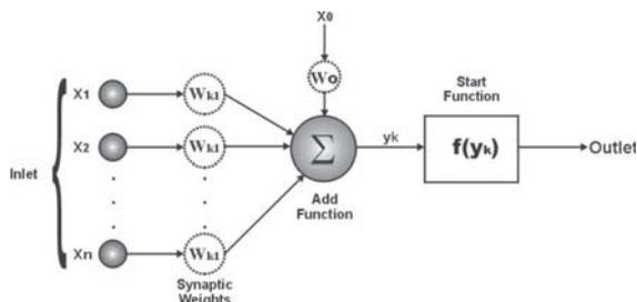
Figure 1 - Rosenblatt's Model of Artificial Neuron
