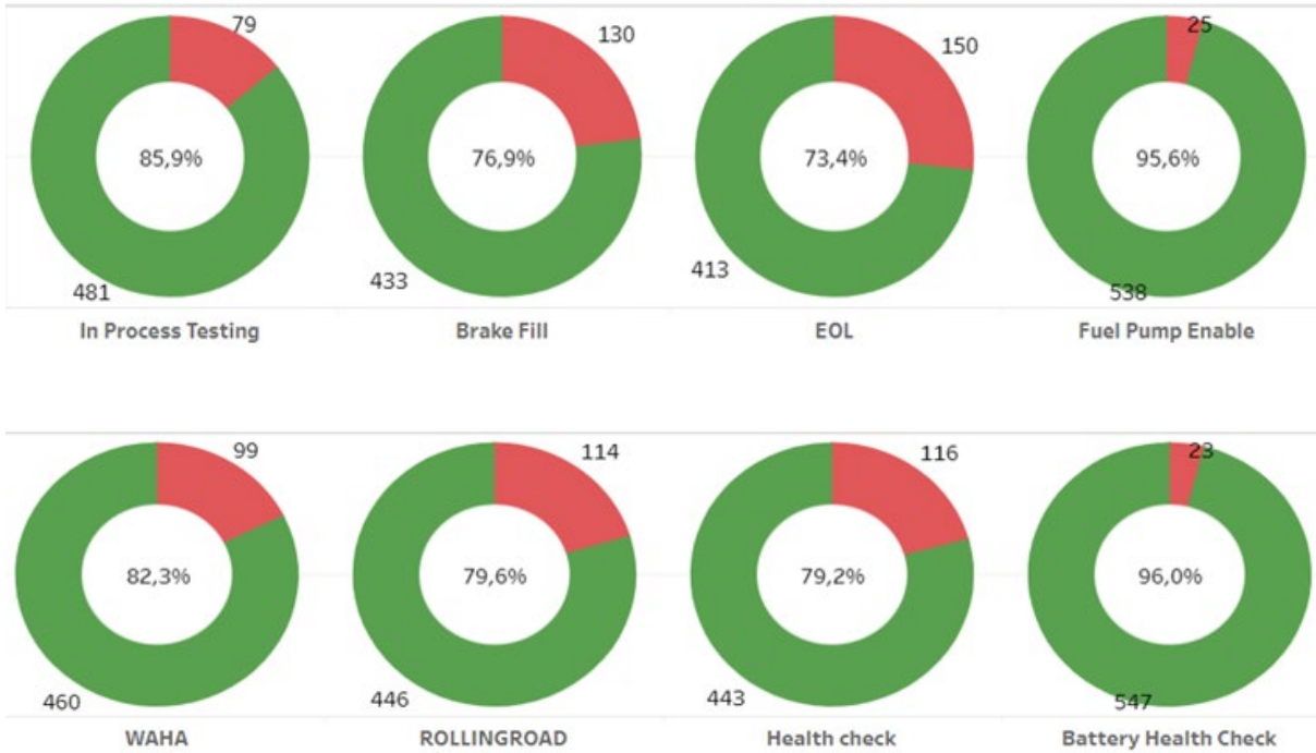
Figure 7 | RFT indicator by electrical parameterization station after applying the algorithms.
